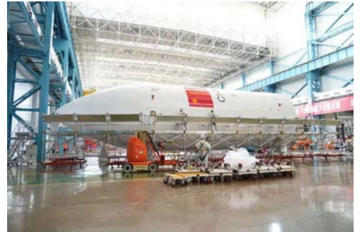
Feb 2023: Extended Fairing Under Construction in Tianjin
