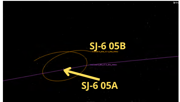
Mar 2022: SJ-6 05B & SJ-6 05A operated so close to one another that TLE measurements can't give an idea of which satellite is orbiting the other (LSAS)
