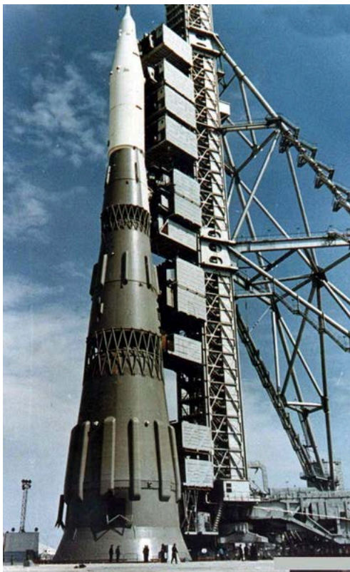
November 23rd is the anniversary of the 4th launch of the Soviet N-1 rocket, which flew until it shut down 6 engines to reduce stress. Shutting those down caused a fluid hammer which ruptured the plumbing causing a fire. ( @DJSnM via X)
