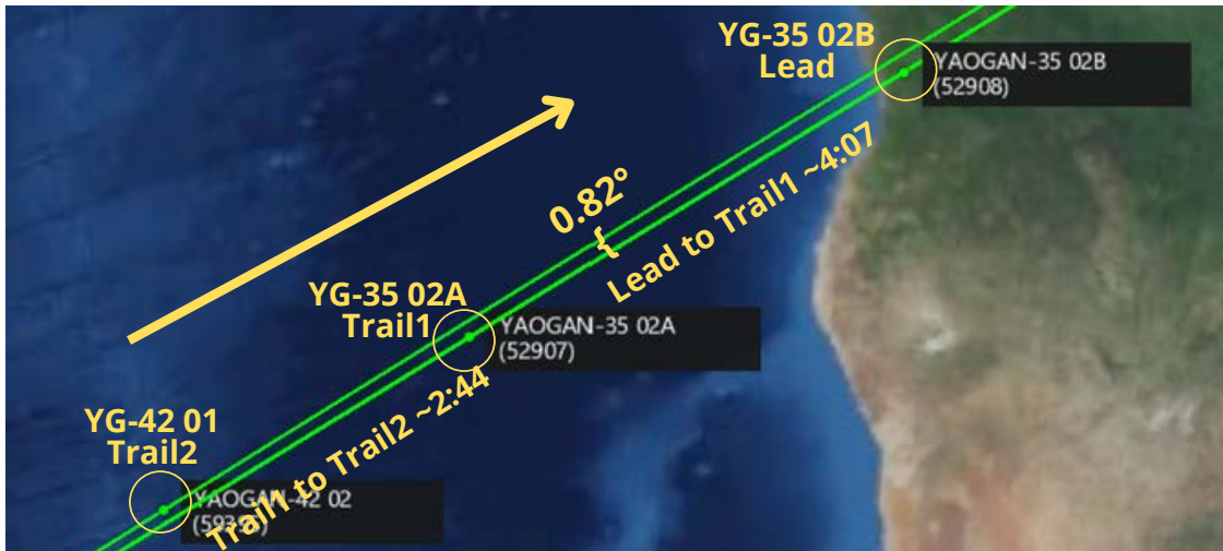
YG-35 02 Example of Narrow RAAN Offset (0.82° West) Between Lead/Trail1 and Trail2 (spaceaware.io)
