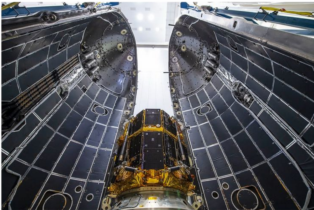
HAKUTO-R Mission 1 lunar lander encapsulated inside the payload fairing of the Falcon 9 rocket
