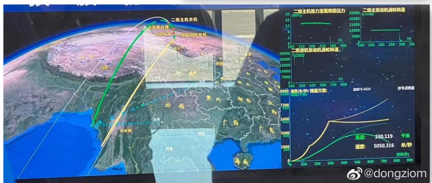
Screen Shot from Mission Control Center Indicates Problems with 2nd Stage Vernier Engines
