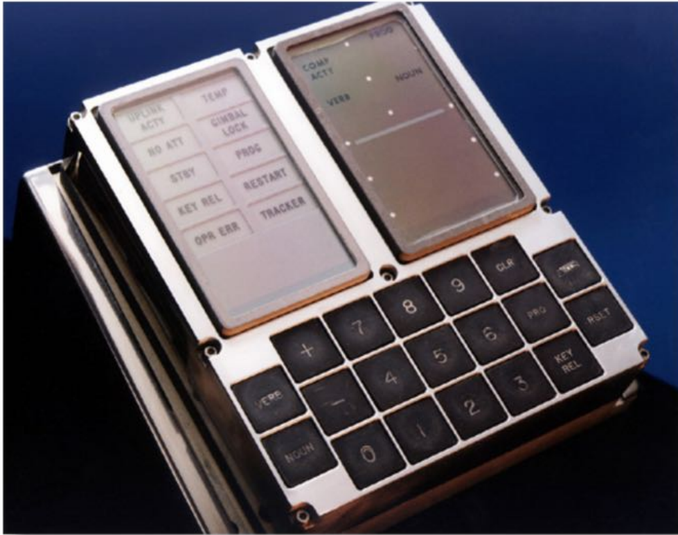
Apollo Guidance Computer - a marvel of 1960s technology, Running at 0.043 MHz (typical laptop > 2000 MHz).
