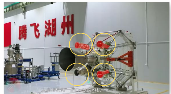
Model of 2nd Stage Propulsion System with Highlighted Vernier Engines
