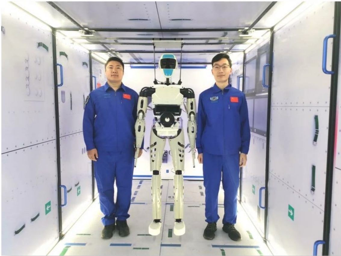
Meet Taikobot, the robot for Tiangong Space Station (CSS). It's designed for station maintenance and astronaut assistance. It is 1.71m tall, weighs 25kg, and has 54 degrees of freedom in total
