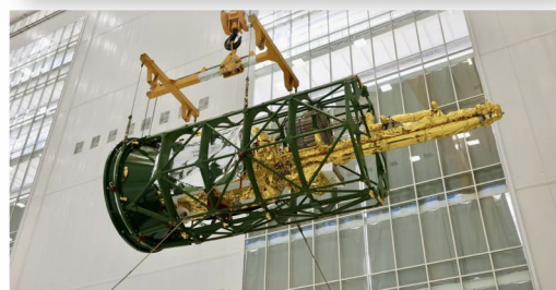
Kondor in Protective Cage & attached to Briz Upper Stage
