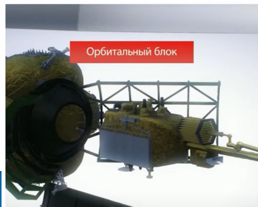
Rendering of Kondor Deployment... Upper Stage Remains Attached to Briz Upper Stage
