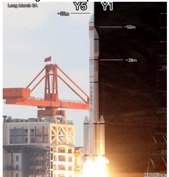
Comparison between LM 6A Y5 and Y1 shows Y5 has a special long fairing that makes it taller, nearly 55m tall while Y1 and Y2 were about 50m
