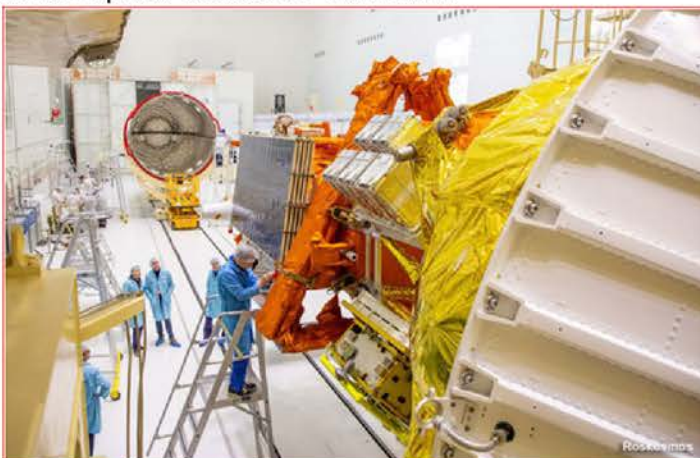
Ride-along Cubesats Mounted Between Fregat & Meteor M2-4 (russianspaceweb.com)
