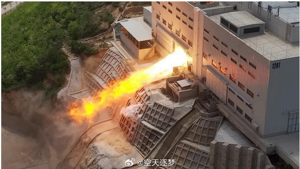
China (CASC) Tests Four YF-100K engines. The YF-100K engines make up the first stage of the Long March 12, a new rocket to debut in 2024 (@CNSpaceflight via X)
