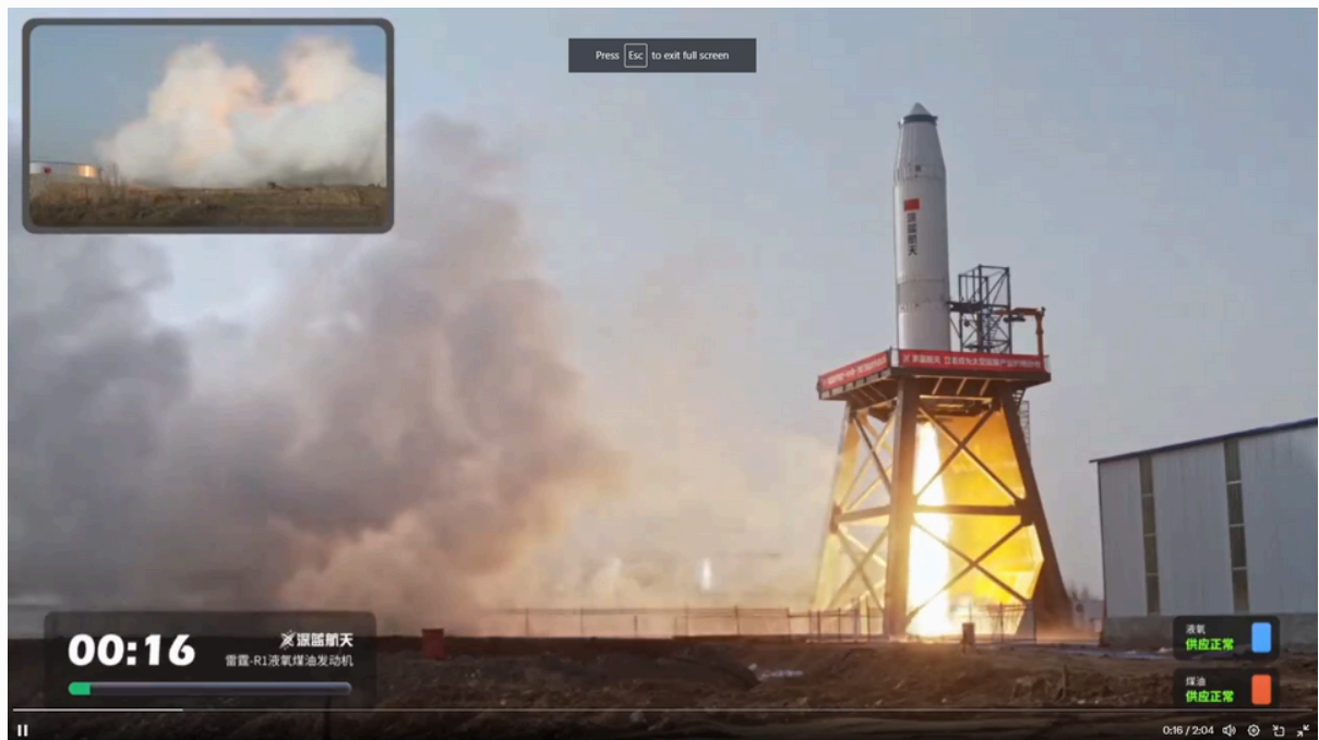
Chinese Commercial Space Company DEEP-BLUE completed a 215 second hot fire test of their Nebula-1 Vertical Take Off/Vertical Landing hopper (@CNSpaceflight via X)
